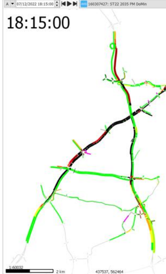
Figure 15. Average delay for evening peak – 2030, 2035, and 2040 Do Minimum Scenario
