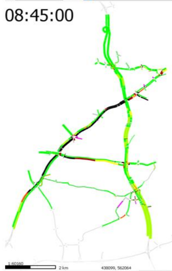
Figure 13. Average delay for morning peak – 2030, 2035, and 2040 Do Minimum Scenario
