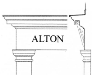
Discreet strip lighting concealed underneath the cornice.
