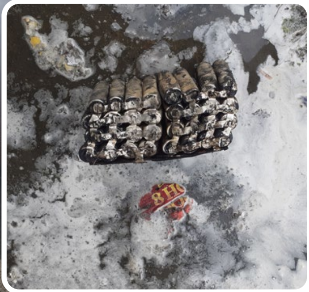
Fires in refuse vehicles caused by batteries
