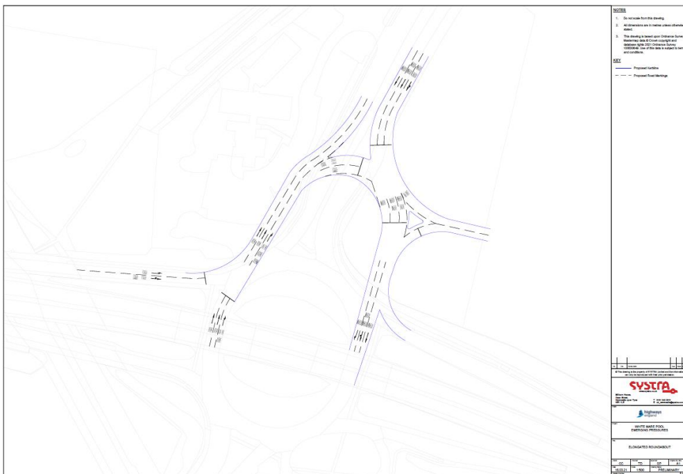
Figure 2.2 Elongated roundabout at White Mare Pool
